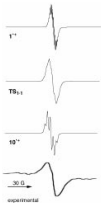
Figure 2. Comparison of the simulated ESR spectra for 1^+ , TS_{1-1} , and 10^+ (0 K) at BCCD(T)/cc-pVDZ with the experimental ESR spectrum for 1^+ (77 K, bottom, scanned from ref. [11] with permission). TS_{1-1} represents the averaged spectrum for rapidly interconverting, degenerate isomers of 1^+ .
